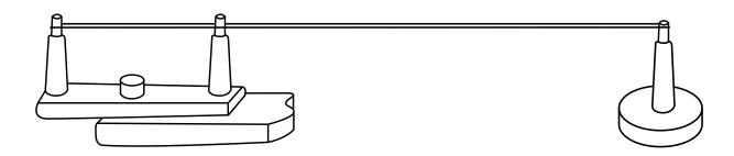
A simple portable wooden string jig can be clamped onto a table or work bench.
