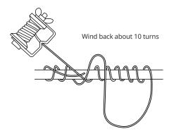
Then, start wrapping the bottom loop to tighten and wrap the serving on the left hand side. The loops on the right side will unwrap as the left side wraps. When this is done, pull the string with the server to take up the slack.
